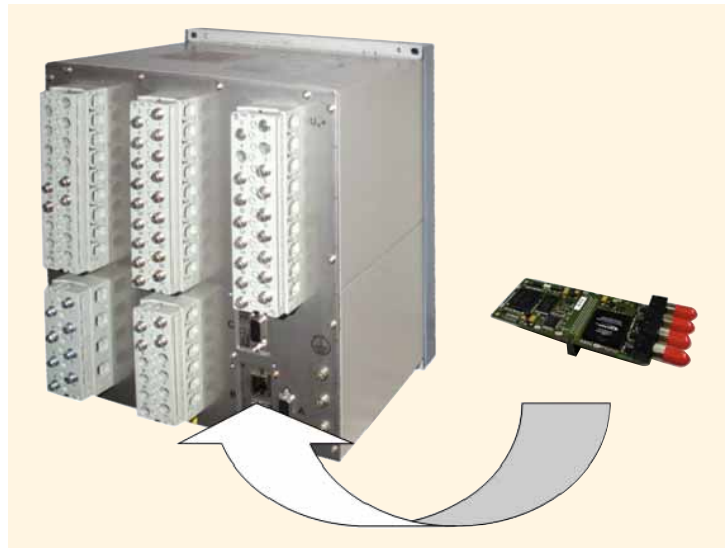
Fig. 28 Upgrading an existing IED with IEC 61850 communication
