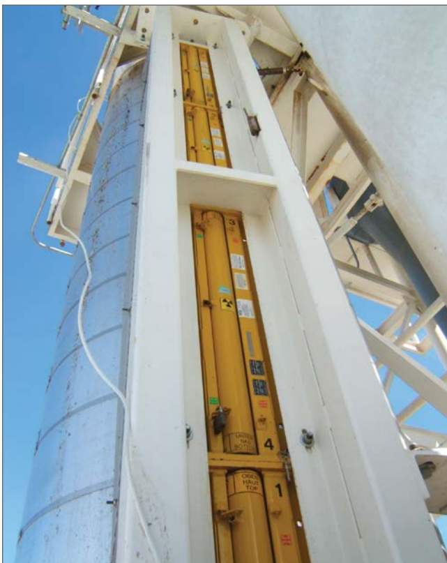
CONTINUOUS LEVEL GAUGE ON TOMATO-FILLED COLUMN
