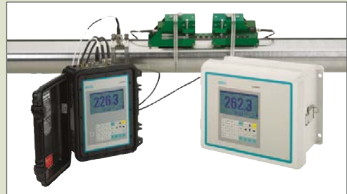
Figure 1. By measuring the difference in the speed of sound transmitted and received (transit time), these ultrasonic meters measure velocity and compute flow.
