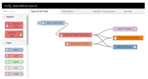
A Node-RED flow uses prebuilt nodes to make programming the IIoT easier.
