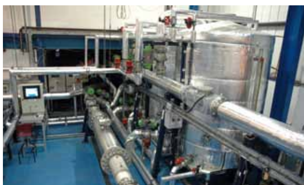
Figure 5.1: Calibration for large-size Coriolis measuring devices
