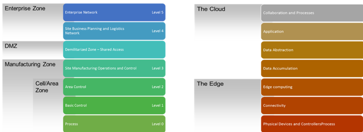
Figure 3 Purdue Enterprise Reference Architecture model on the left and IoT Reference Model on the right
