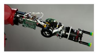
47-pound arm goes into zero gravity mode – making it virtually weightless. The SEA is what gives Baxter its unique smoothness of handling and ensures it won't damage parts, fixtures, materials or people.
