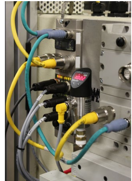
Figure 10: EtherNet/IP IO-Link Master with smart pressure sensor
